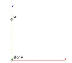
• After placing the last point, type **3** into the **L** (Length) field and **95** into the **A** (Angle) field. This gives necessary line size.
