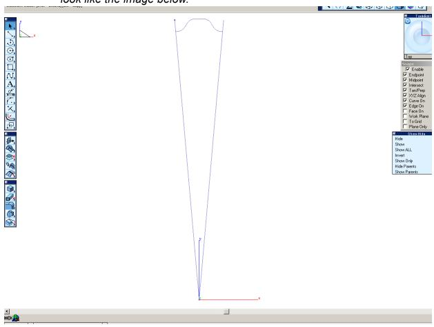
Once all of the fillets are completed, the tooth should be rounded out and look like the image below.
