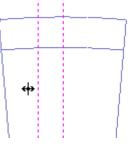
• Next, do the same thing for the right side. Drag a new line off of the center construction line or just enter a negative value in the status line (-.10), and press the ENTER key and a new construction line is created.
