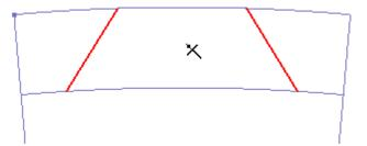
• Select the parts of the arcs to be trimmed away. On the upper arc select the two parts outside of the two line. On the inner arc, select the part inside the two lines. The tooth should be similar to the one below.
