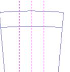
Create one parallel line off of the original. The rest of the lines can be created by entering different + & - offset values into the Status Line data box.
