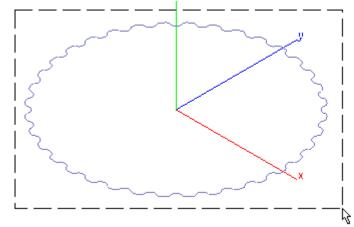
• Now it needs a direction to extrude the profile. Select the origin for the first point and straight up along the *z*-axis for the second.
